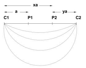
Figure 4.1: Simple array for resistance survey
